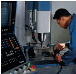
Production moulds are manufactured using modern CNC machine-tools.
