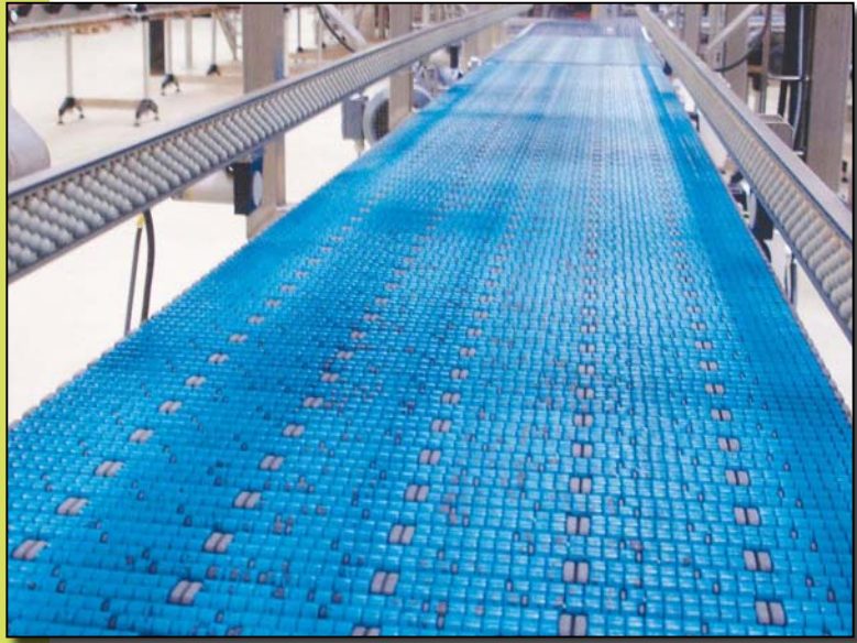
CONVEYOR FOR TRAYS WITH CANS.
