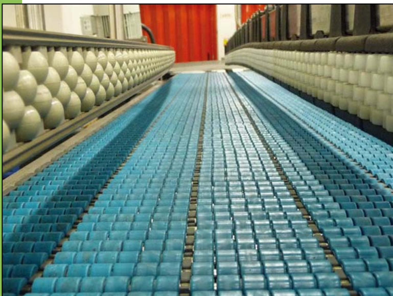
ACCUMULATION SYSTEM FOR SHRINK WRAPPED PRODUCTS.
