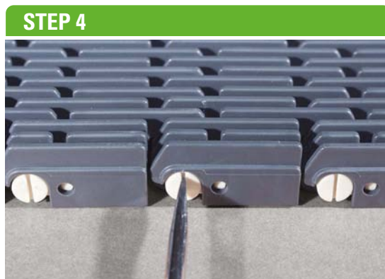
4 - Clip completely rotated. The belt is now closed.
