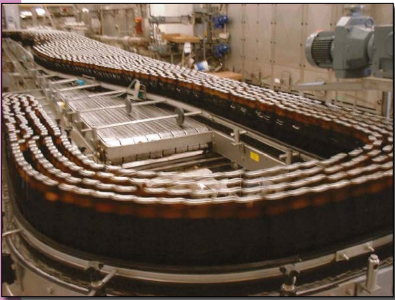
SPEEDLINE STAINLESS STEEL CHAINS IN COMBINATION WITH MAGNETIC CURVES.
