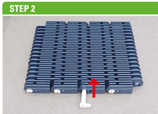
2 - Insert the pin-clip inside the hinge. Push till end position following red arrow direction.
