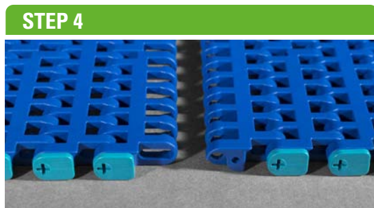
2 - The clip is pushed off after screwdriver rotation.
