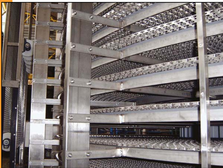
BAR CAP PROFILES FOR SPIRAL CONVEYOR SYSTEMS.
