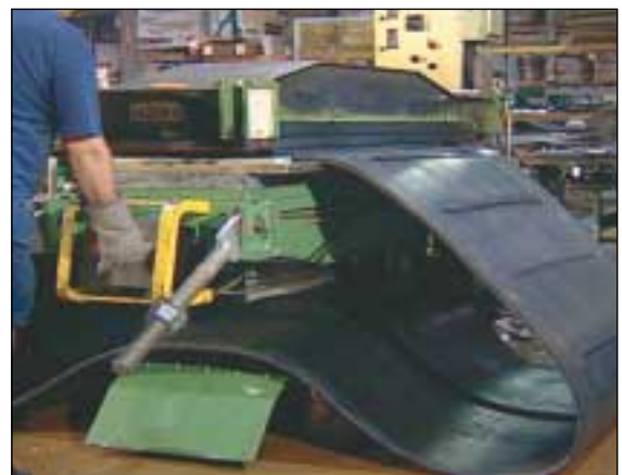
In addition to special heat presses, vulcanization requires a thorough knowledge of vulcanization solvents and other chemicals. It is also a time-consuming process.
